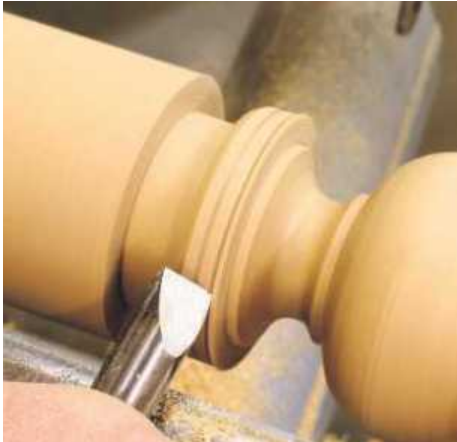
▲ Pic.19 Some people see the skew chisel as the ultimate in turning tools. Here I am using a 10mm round version to cut this bead at the top, but switch to a gouge if you are more confident using that tool
